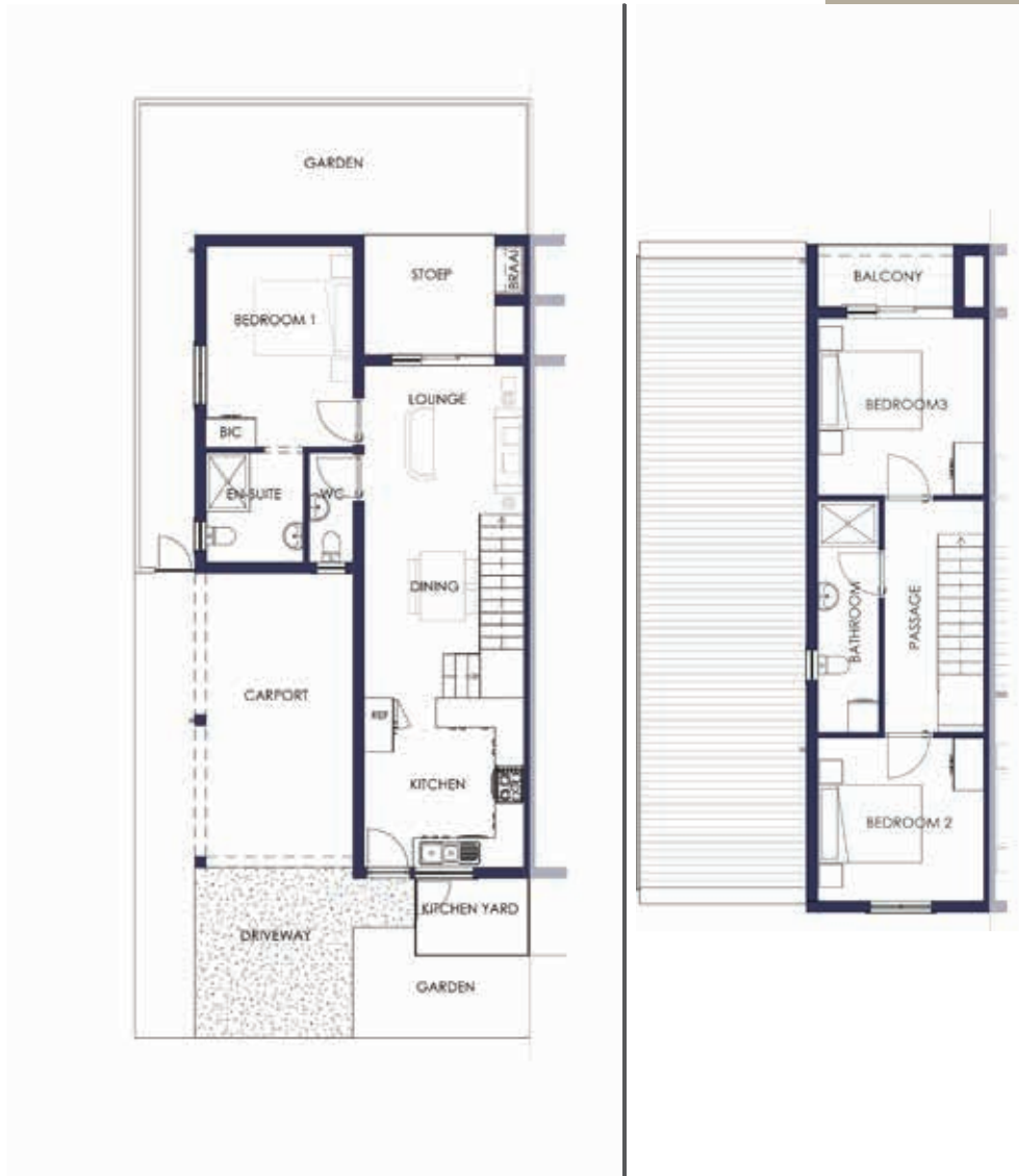
Ground Floor First Floor
